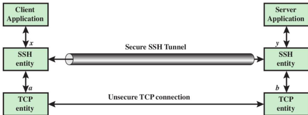
$x$  and  $y$  are application port numbers,  $a$  and  $b$  are port numbers used by SSH
