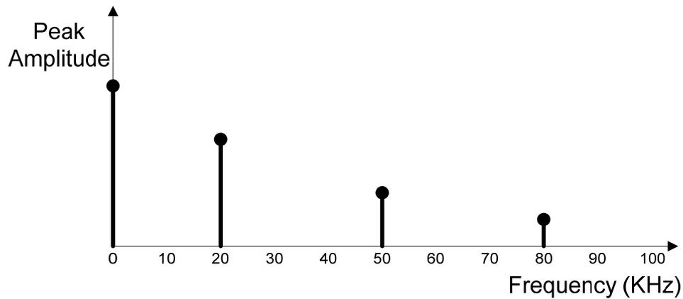
**Figure 2: Analog signal in frequency domain**
