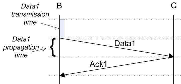
**Figure 5: B to C using Stop and Wait**
