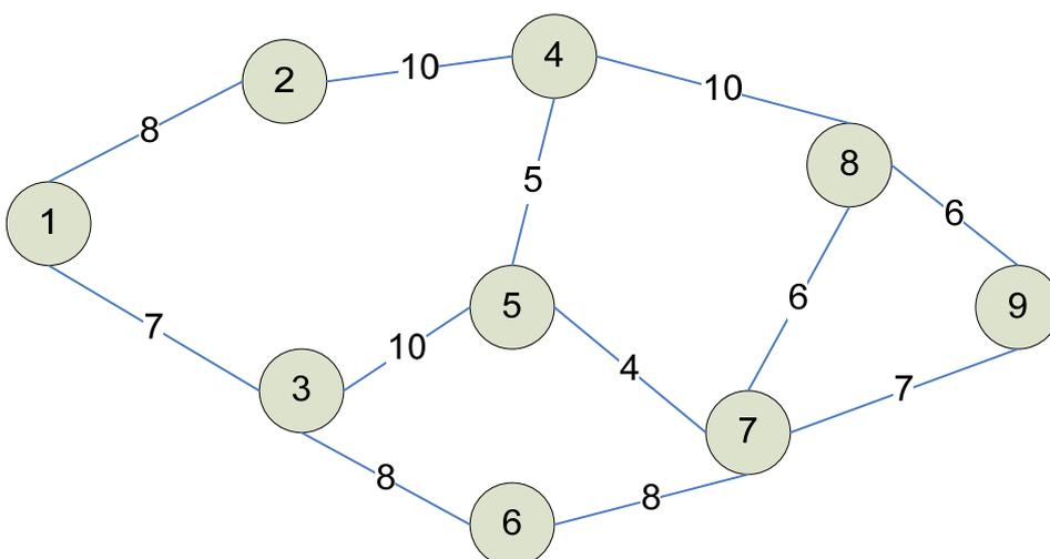
Now if the criteria for selecting a path (or route) is based entirely on the maximum capacity, then what path would be selected? In other words, what path should be based to allow for the highest amount of traffic to be sent from node 1 to node 9?
