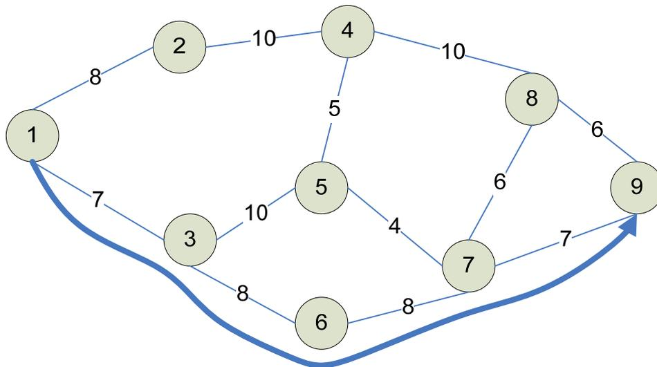
Why this path? Because using this path we could potentially maintain a data rate of up to 7Mb/s. The minimum link capacity along the path is 7Mb/s (the maximum is 8Mb/s). The minimum link capacity determines the maximum path capacity.
