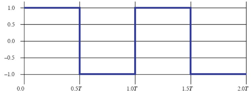
$$s(t) = \frac{4}{\pi} \sum \frac{1}{k} \sin(2\pi(kf)t), \text{ for } k \text{ odd}$$
