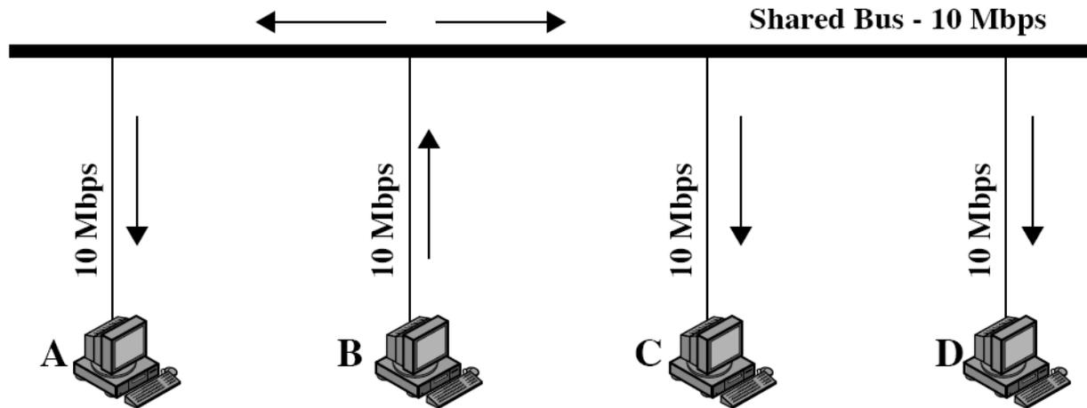
Ethernet in Bus Topology: only one station can transmit at a time (because a transmission goes everywhere on the bus) therefore stations must share the LAN capacity. Each station gets 2.5Mb/s
