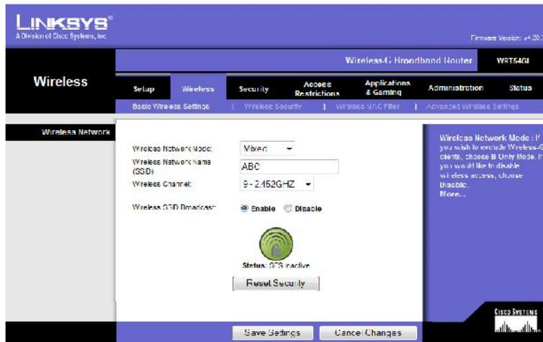
**Figure 2: Linksys WRT54GL Wireless Router Configuration (Wireless Tab)**
