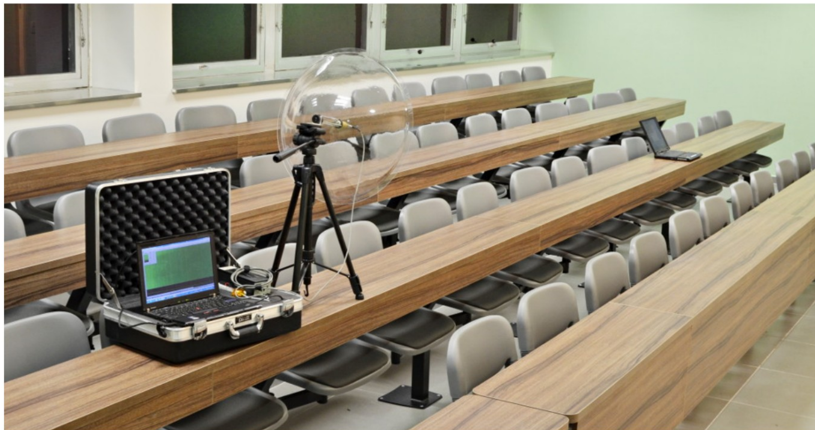
Figure 6: Parabolic microphone (same as in Figure 5), attached to the portable measurement setup (in a padded briefcase), attacking a target laptop from a distance of 4 meters. Full key extraction is possible in this configuration and distance (see Section 5.4).
